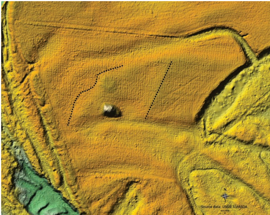
Figure 5. Lidar image of 3DA673 site vicinity; dotted lines indicate locations of linear magnetic signatures from gradiometry survey.
