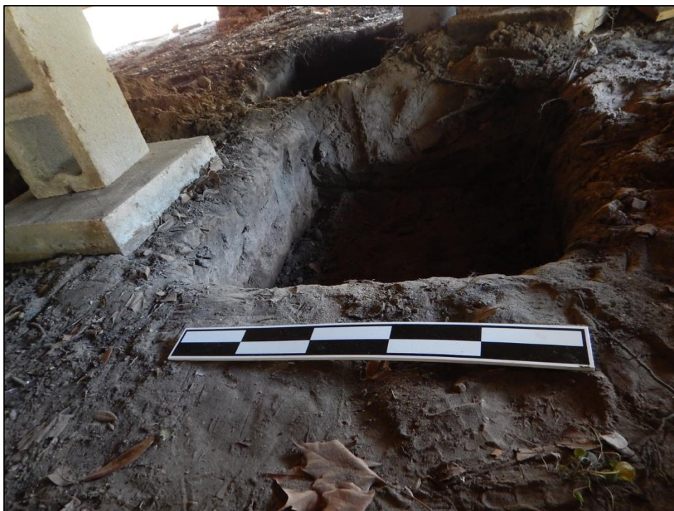
Figure 5-16. Hand excavated pier located near an existing pier, on the western side of the house.
