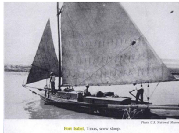
Figure 3-2. A historic photograph (date unknown) showing a Texas scow sloop underway (as presented in Chappelle 1951:175).
