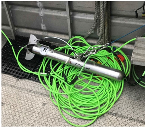
Figure 4-5. EdgeTech 4125 dual frequency side-scan sonar system.
