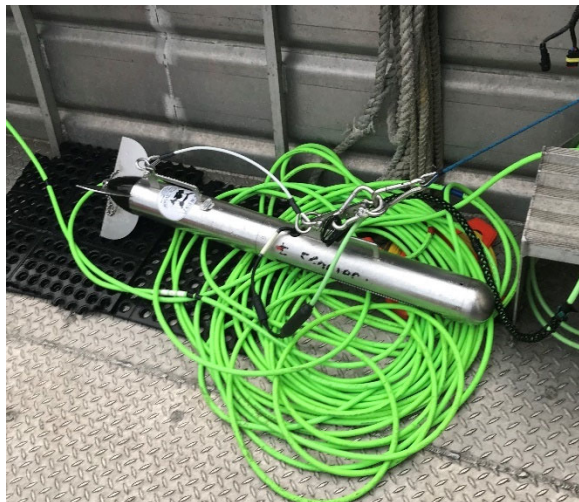
Figure 4-3. EdgeTech 4125 dual frequency side-scan sonar system.
