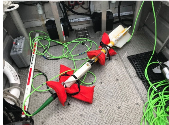
Figure 4-5. Geometrics G-882 Marine Magnetometer with life preservers attached for towing in shallow water.
