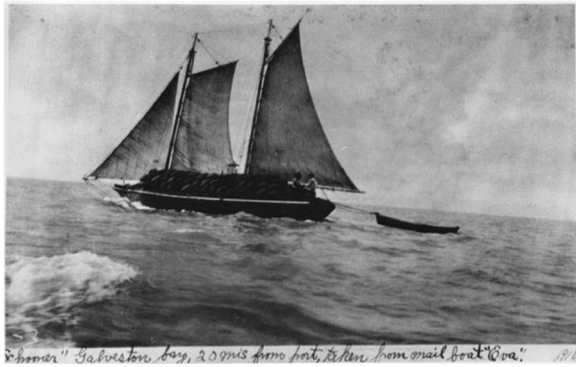
Figure 3-1. Photograph taken in 1910 on Galveston Bay showing a two-masted scow schooner in transit loaded with cargo (photograph courtesy: The Portal to Texas History).
