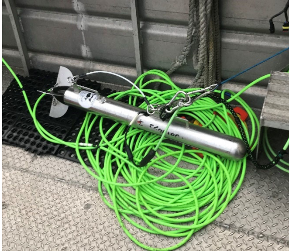
Figure 4-3. EdgeTech 4125 dual frequency side-scan sonar system.
