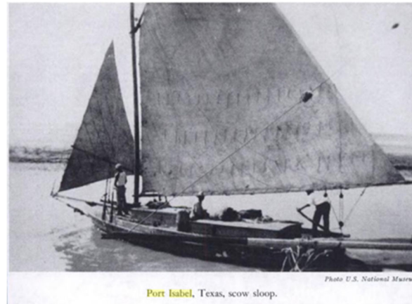
Figure 3-2. A historic photograph (date unknown) showing a Texas scow sloop under way (as presented in Chapelle 1951:175).
