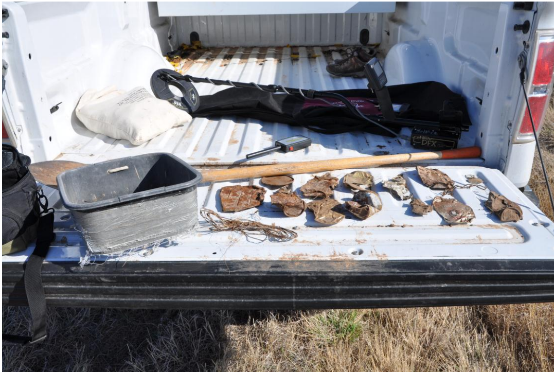
Figure 11. Metal detector survey gear with a sample of recovered modern items from a segment of the survey.
