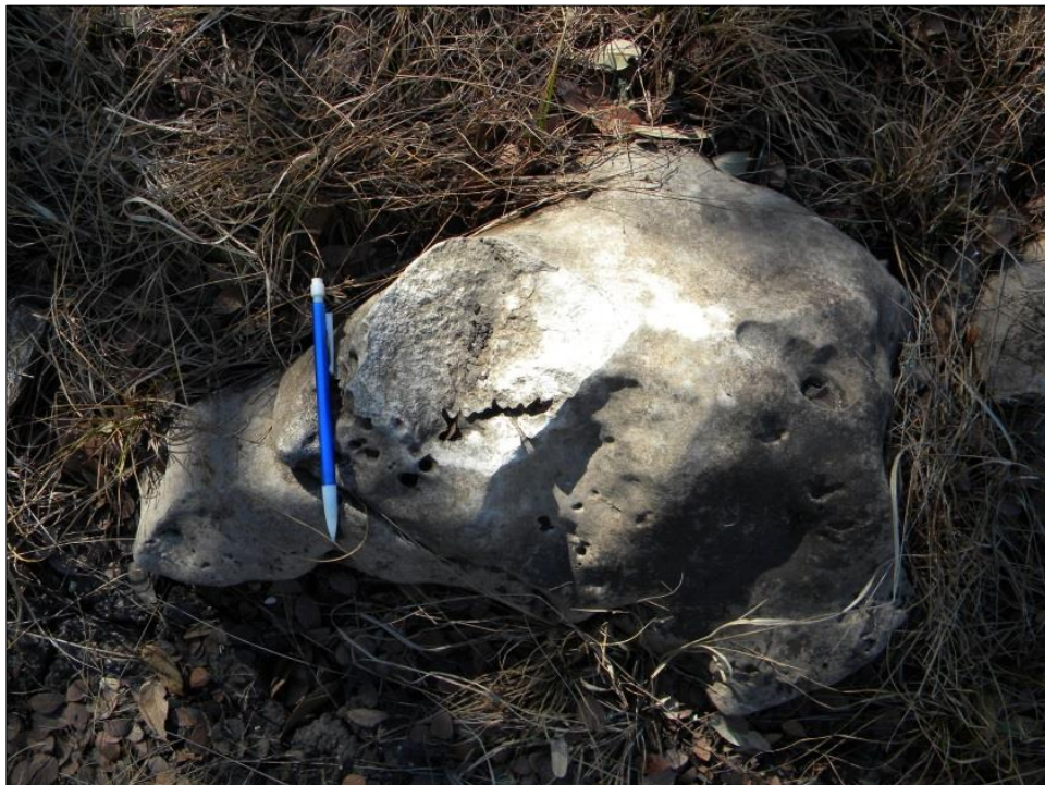
Figure 8. Evidence of impact damage to large limestone cobble.
