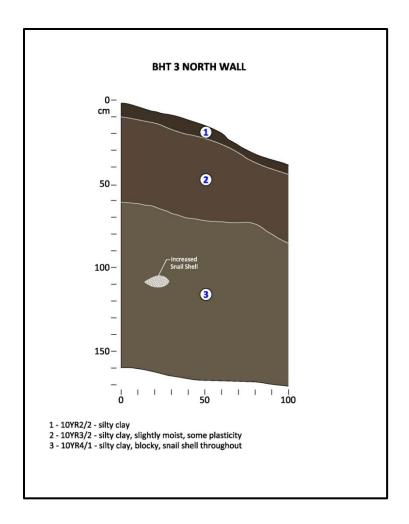
**Figure 5-14**. North wall profile of BHT 3.
