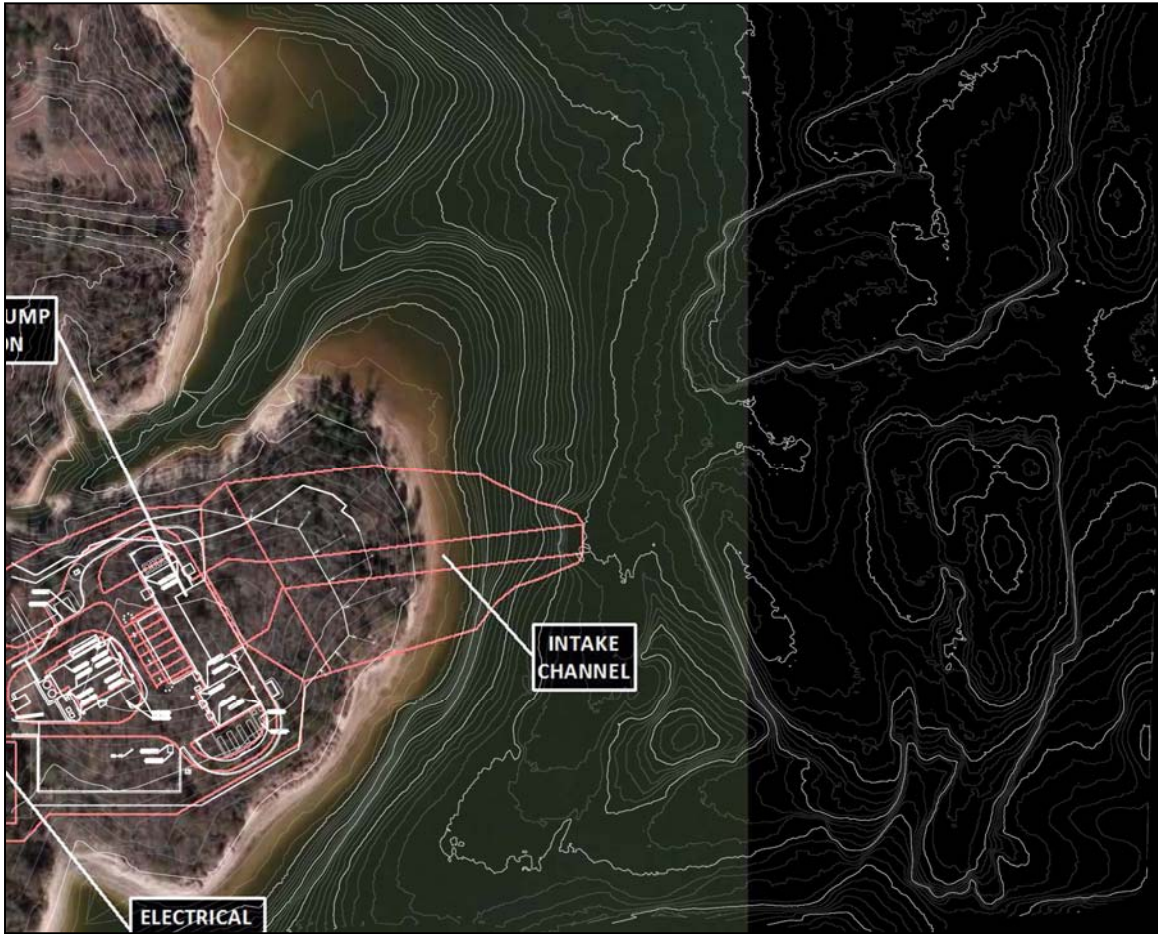
Figure 2. Pump Station Schematics overlaid onto a modern aerial photograph. Bathymetric survey contours offshore are included as well (white).
