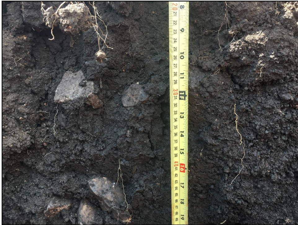
Figure 10. View of dense cobbles and gravels in top stratum of BHT06, north profile.
