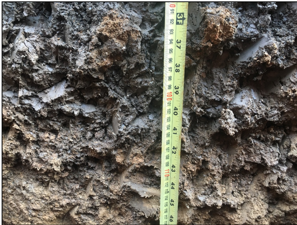
Figure 11. View of transition between strata I and II from BHT05, north profile.
