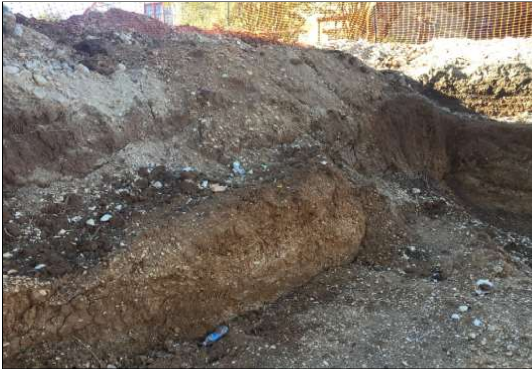
Figure 19. Profile 1 of Alluvial Gravels at Active Construction Site (Facing North)
