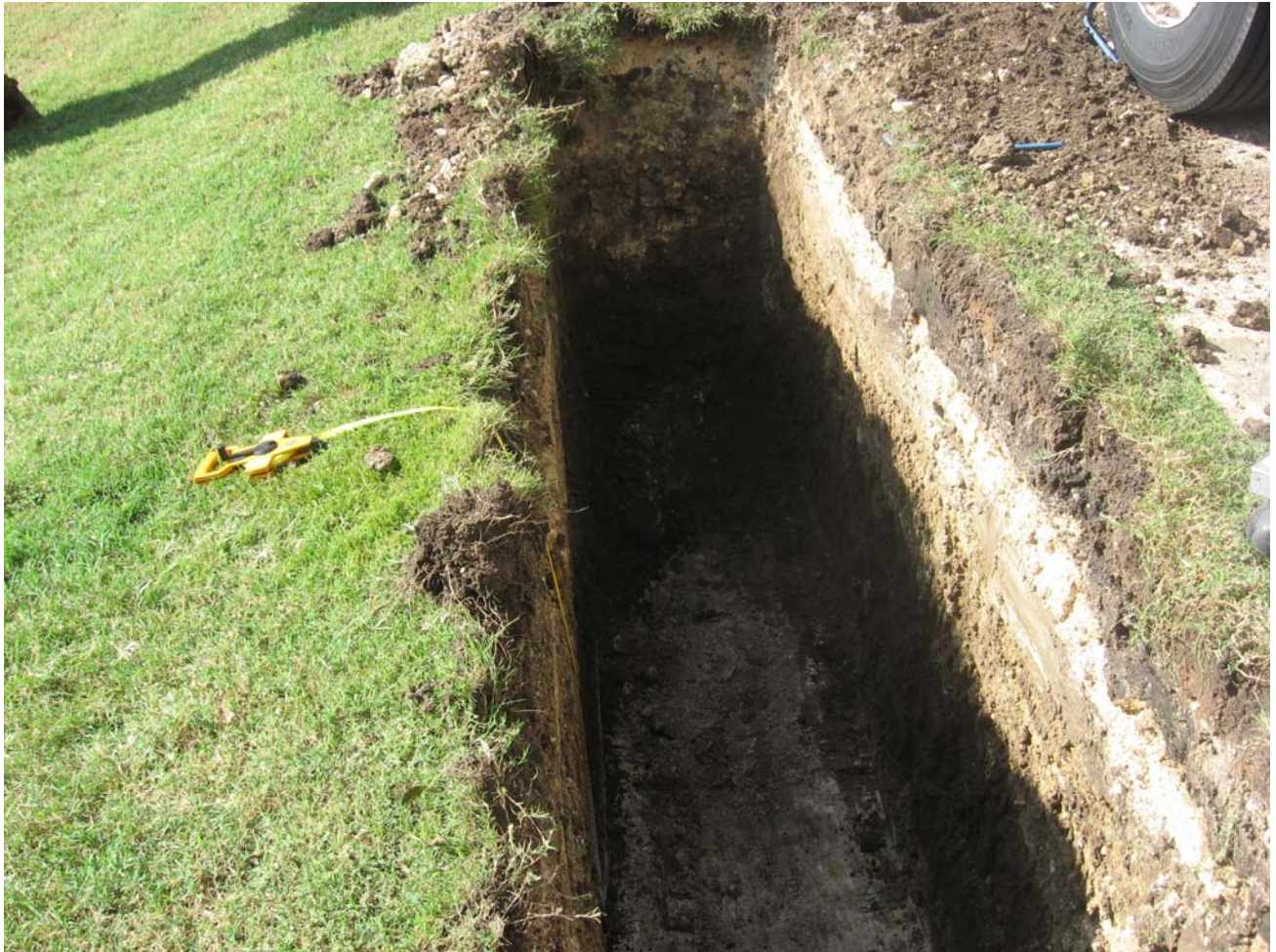
Figure 11: View of GT3, showing the exposure of chalk/marl bedrock at base of trench.
