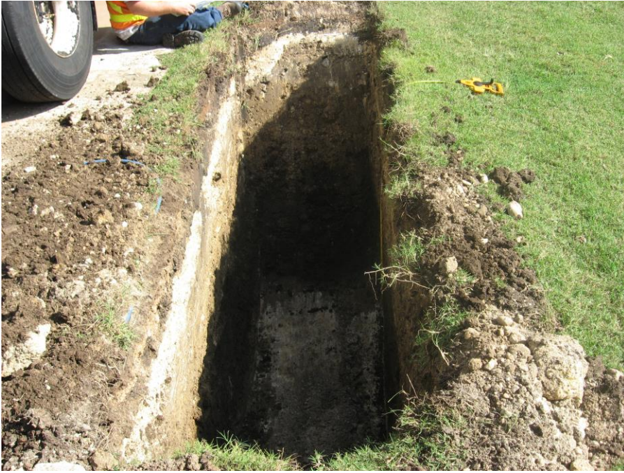
Photo #6: Facing east toward GT #3. Note the chalk bedrock in the bottom of the trench.
