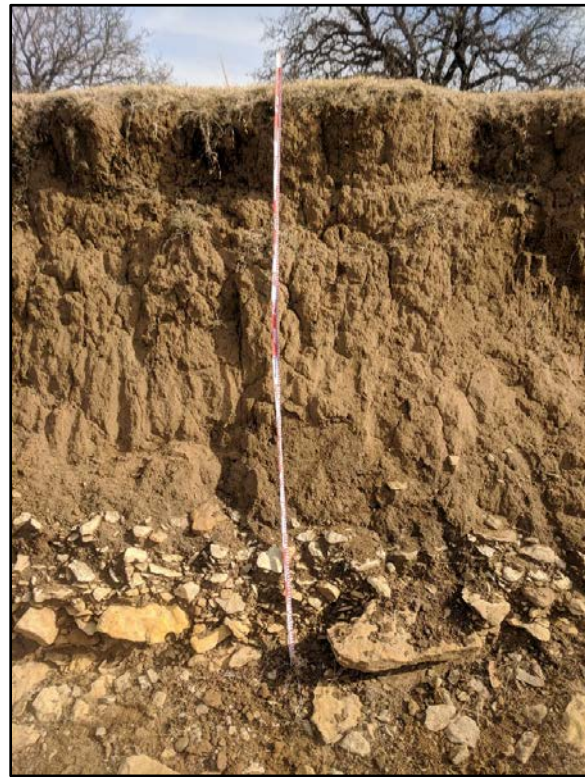
Figure 9. Natural erosional profile in temporary easement in southwestern quadrant, facing west. Note gravels and cobbles at base of profile.
