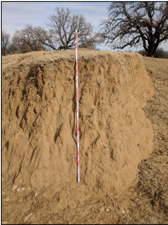
Figure 8. Natural erosional profile in temporary easement in southwestern quadrant, facing west. Note gravels and cobbles at base of profile.
