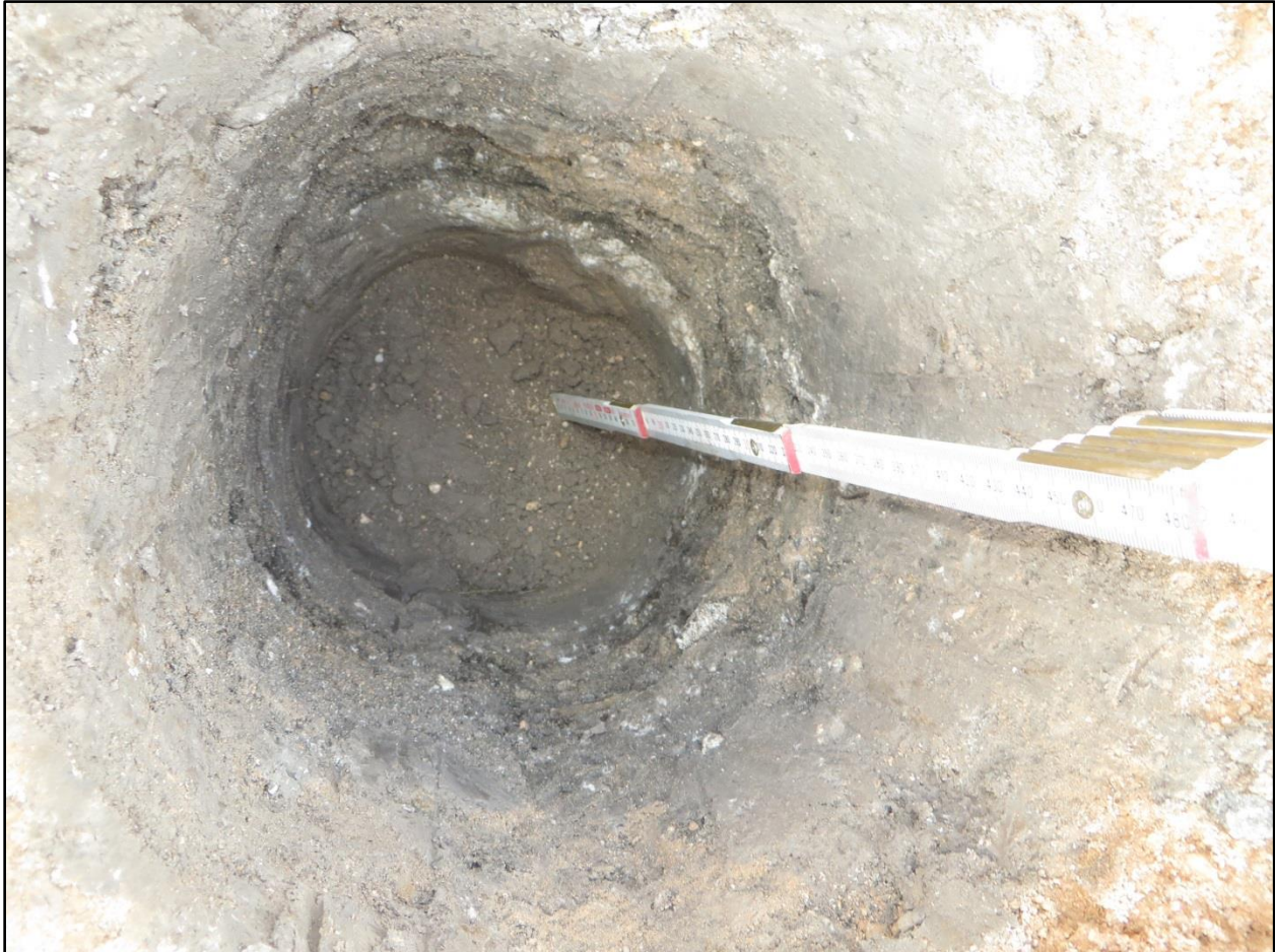
Figure 5-4. ST 3 with tar inclusions in the walls of the profile.
