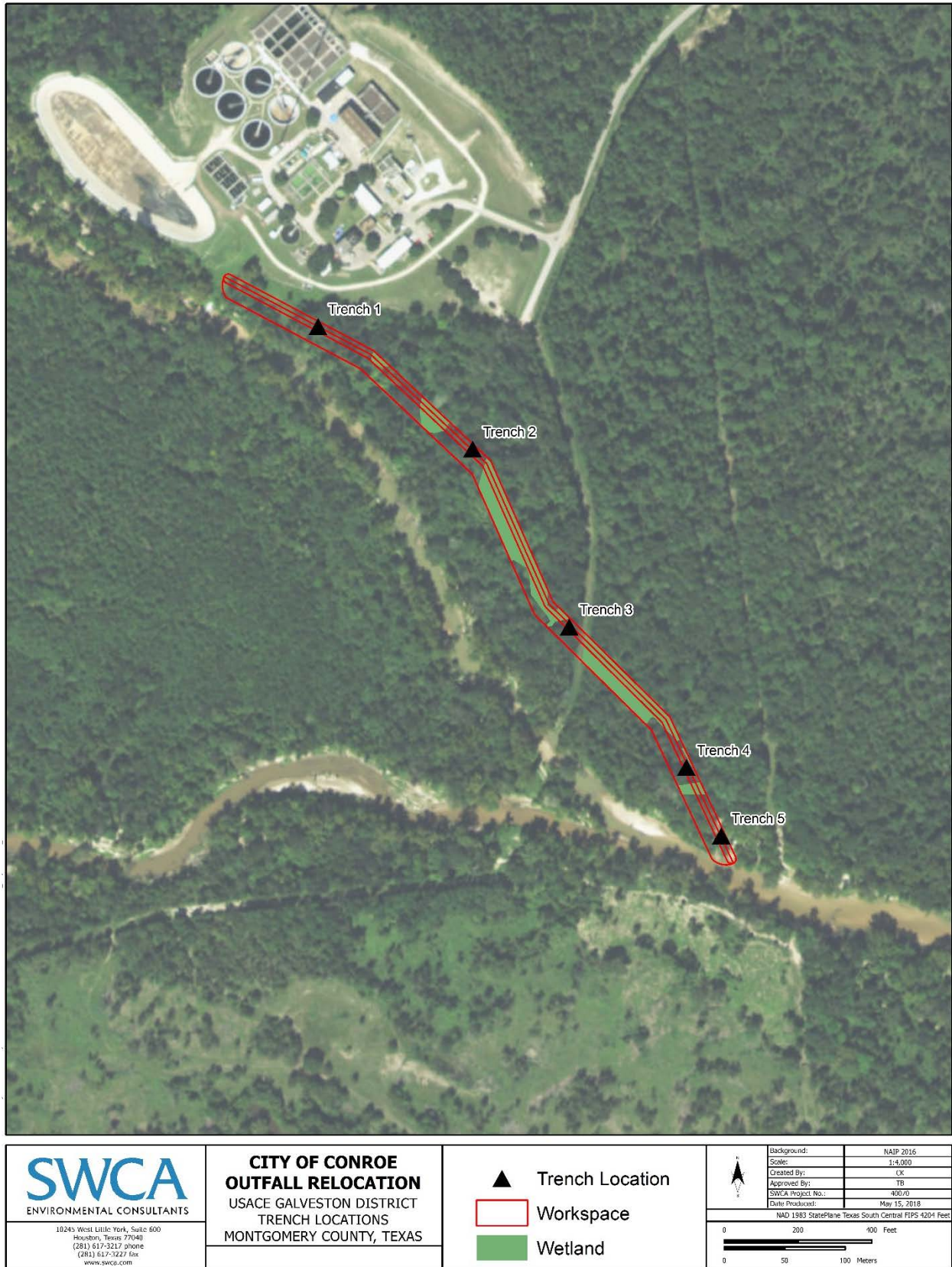
Figure 10. Location of excavated trenches along proposed outfall alignment.
