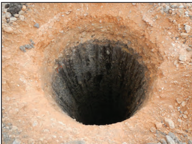
Figure 11.23. Example of soil profile in southern half of substation; Pier 9.
