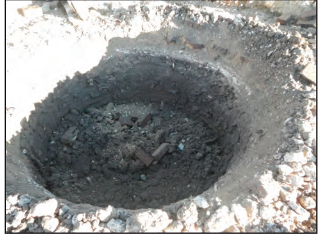
Figure 12.9. Macadamized brick in auger hole and profile of Tower 2 location.
