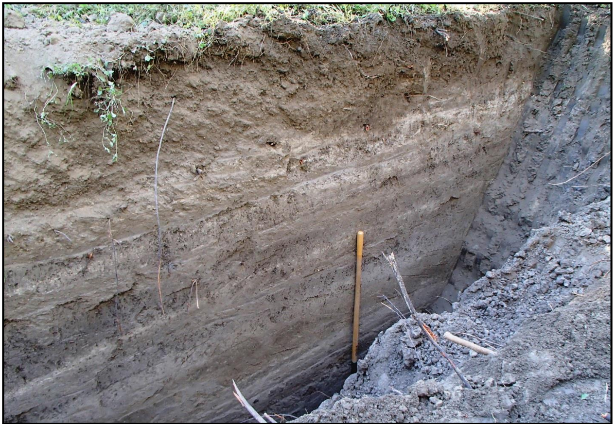
Figure 6-11. Overview of Backhoe Trench 3 profile in lower T_1 terrace depicting multiple zones of stable surfaces (darker zones) and thin flood events (light colors) to a depth of 3 m (12 ft.), view eastward.
