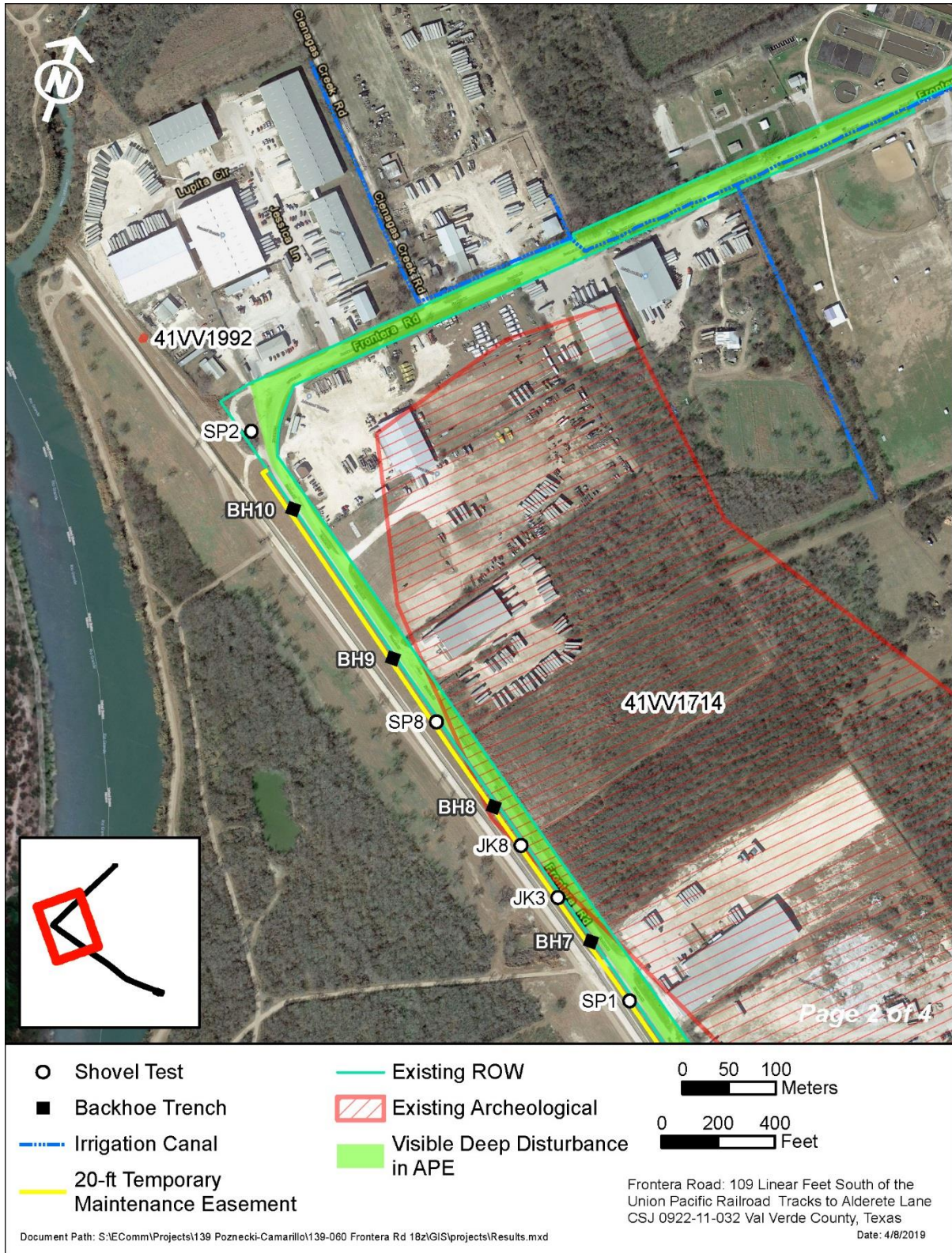
Figure 6. Map of shovel tests and mechanical trenches excavated during fieldwork.
