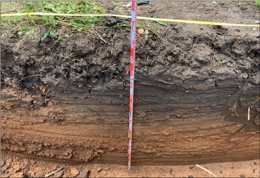
Figure A-4. South Wall Profile of BHT-2
