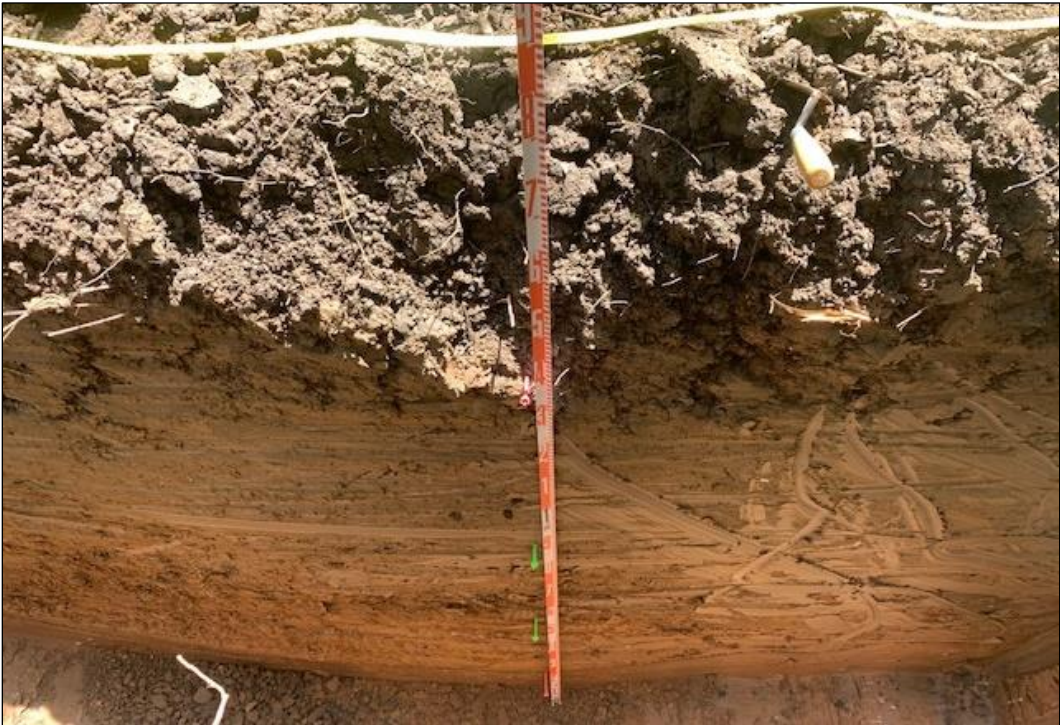
Figure A-10. South Wall Profile of BHT-5
