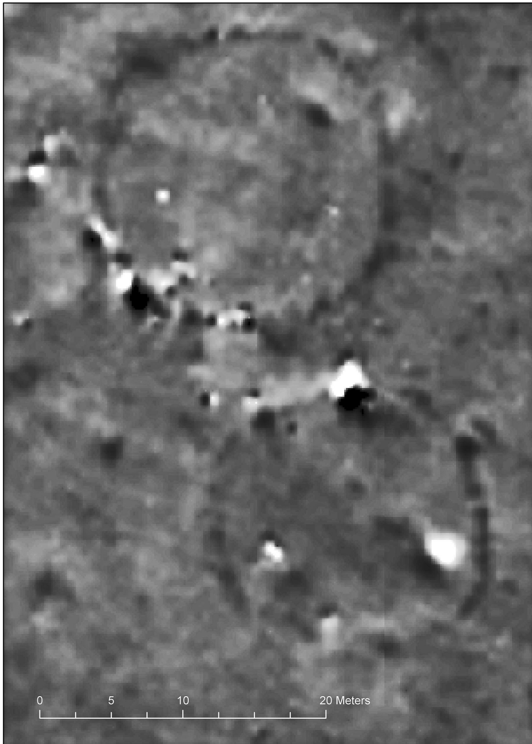
Figure 18. Magnetic features at the George C. Davis site interpreted as rings of postholes.
