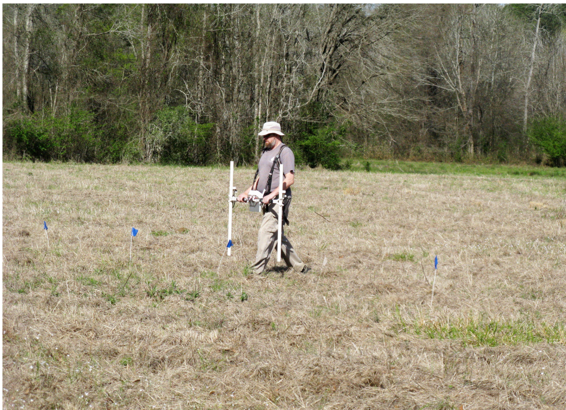
Figure 1. Data collection at Walnut Branch (41CE47) was conducted using a Bartington Grad 601-2 fluxgate gradiometer. White and blue non-metallic pin flags were used to guide the surveyor.
