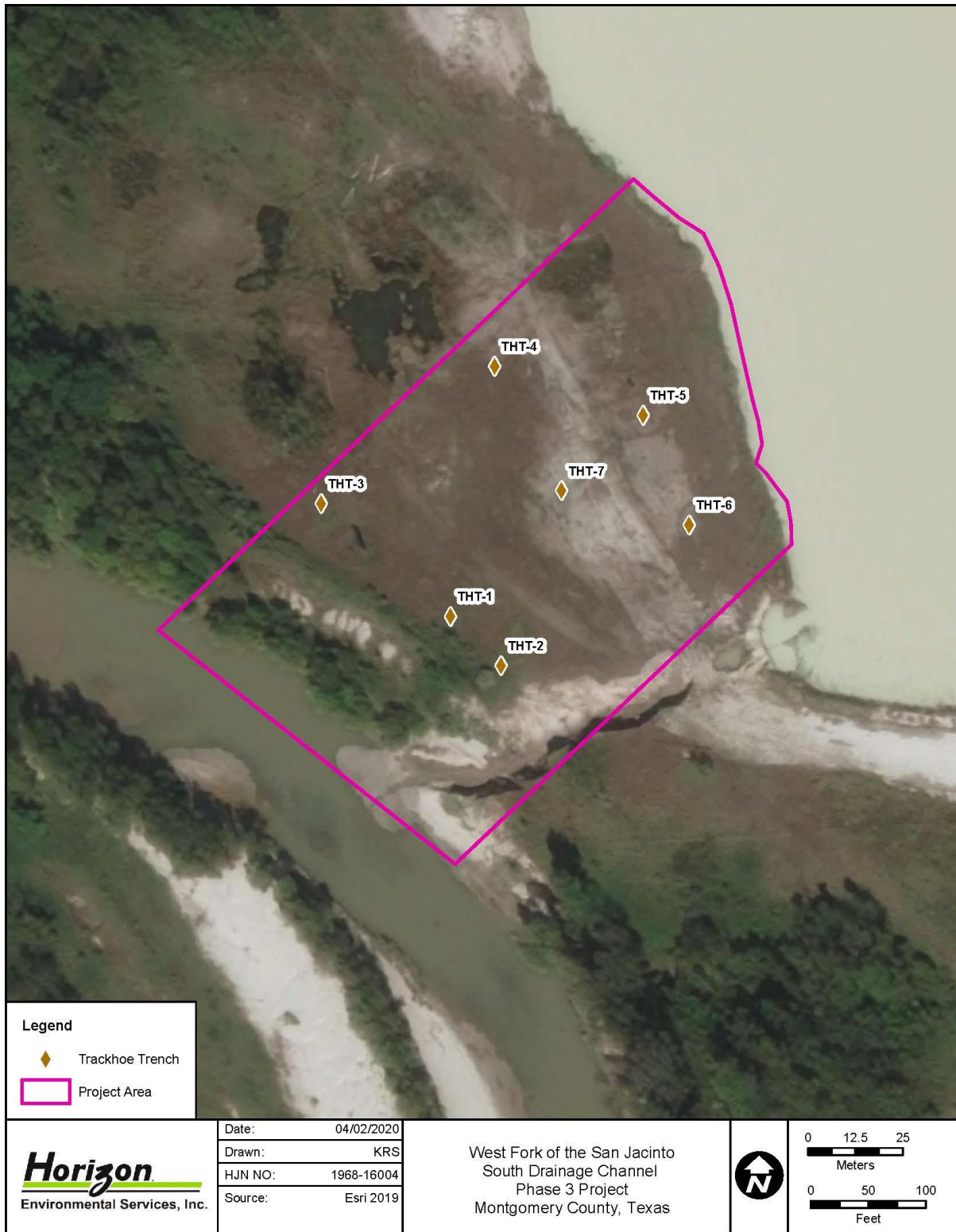
Figure 12. Locations of Trackhoe Trenches Excavated within Project Area
