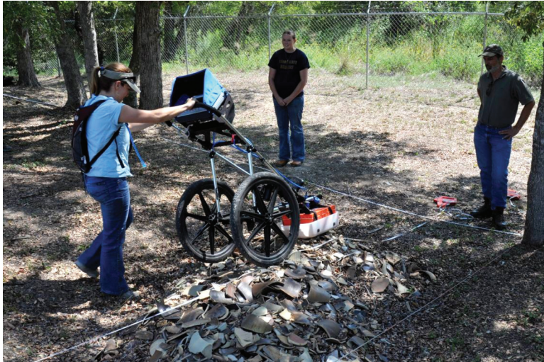
Figure 4-2. Tiffany Osburn conducting GPR survey at the Wilson-Chandler-Durham site. Many obstacles, including this pile of pottery, were encountered across the grid.
