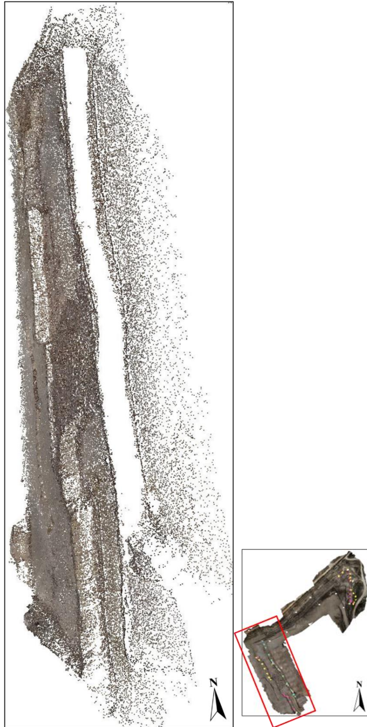
Figure 16: The sparse point cloud model of the Southwest study area, produced in Agisoft Metashape Professional. The first step in the model development process.
