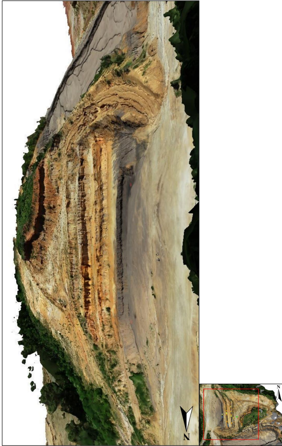
Figure 47: Dense cloud of the Alabama Mine study area in Saline County, Arkansas.
