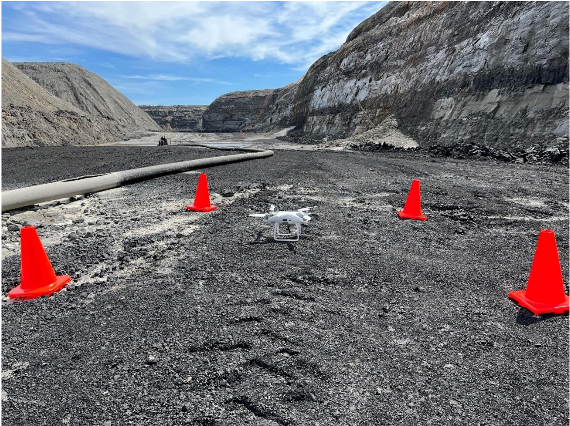
Figure 31: Phantom 4 Pro V2.0 prior to a preprogrammed flight of the study area.
