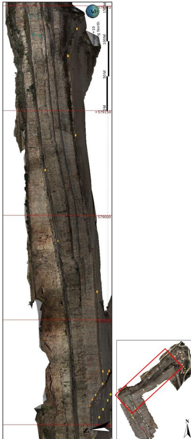
Figure 22: New Braunfels mine composite model viewing the North wall from Leapfrog Geo. This shows a portion of the final model with geologic data points collected from the Geo 7X GPS unit.
