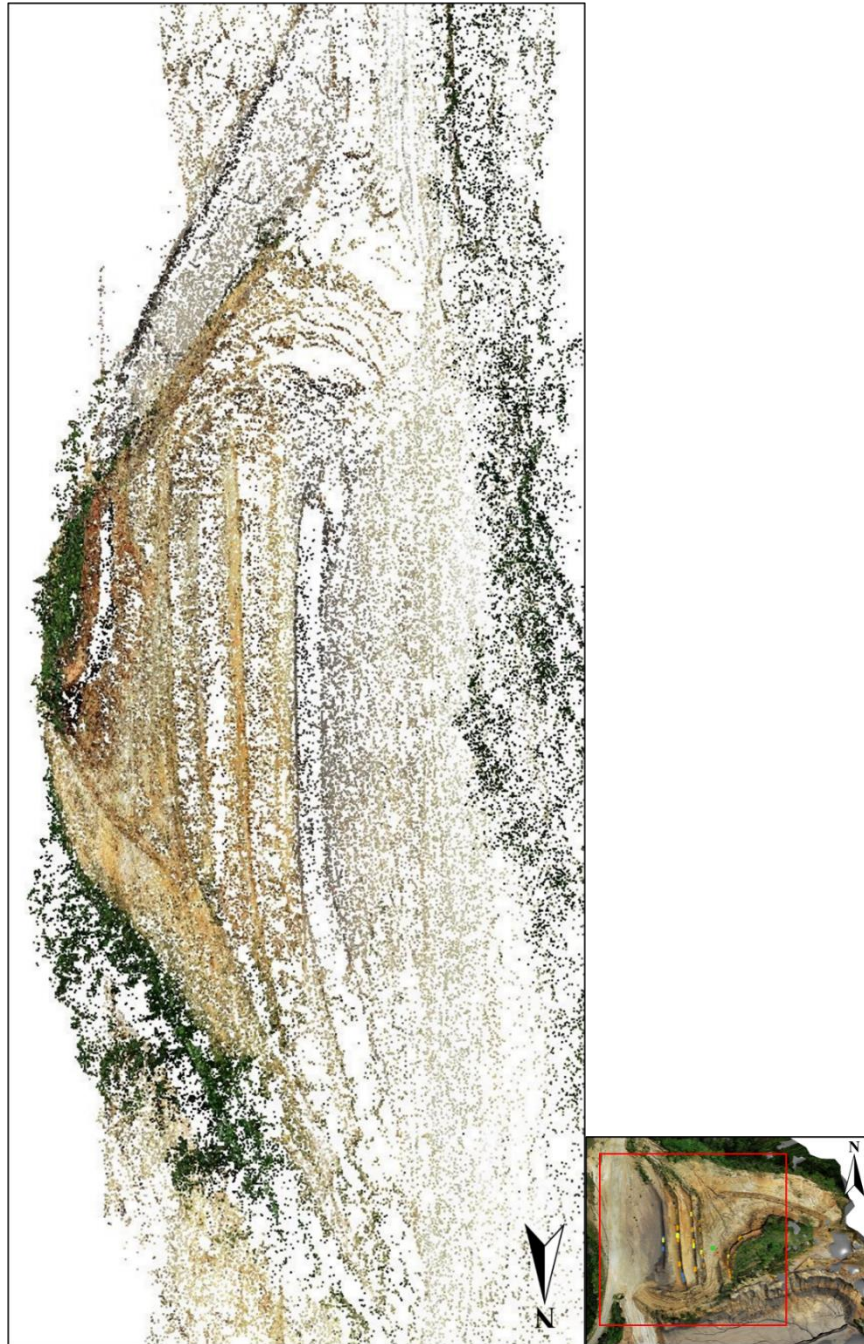
Figure 46: Sparse point cloud the Alabama Mine study area in Saline County, Arkansas.
