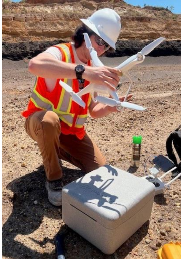
Figure 3: Preparing the DJI Phantom 4 Pro V2.0 for conducting a preprogrammed flight of the study area at the Alabama Mine in Saline County, Arkansas.
