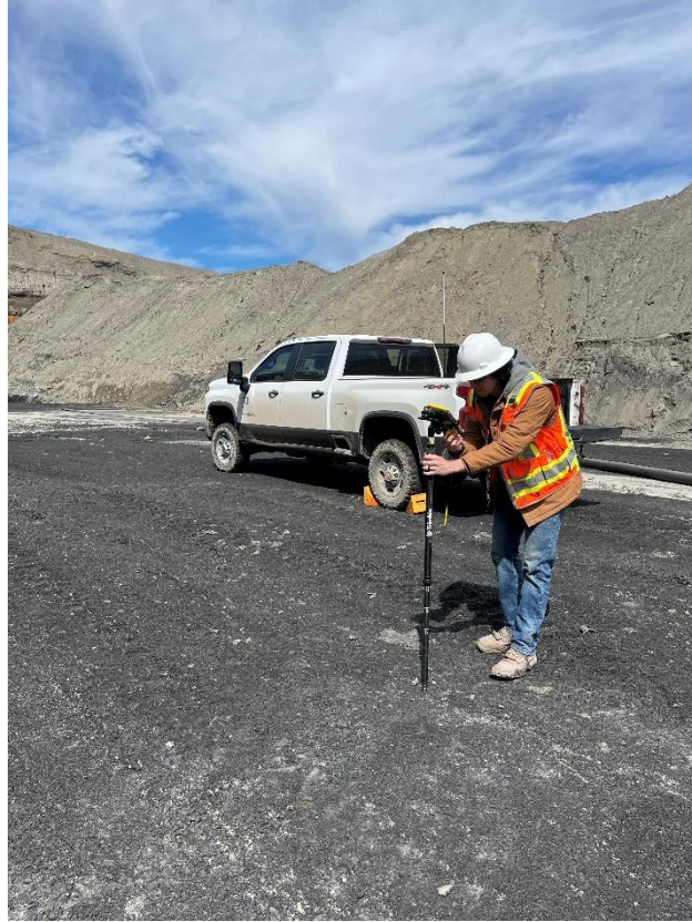
Figure 30: The laser rangefinder on the Trimble™ Geo 7X being used to collect geologic point data along the quarry highwall.
