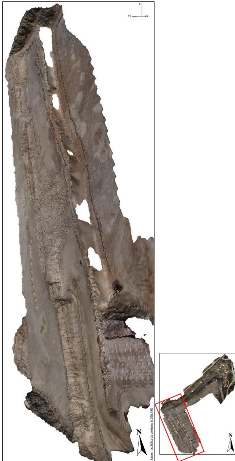
Figure 18: Mesh model of the Southwest study area in Agisoft Metashape Professional. The third step in the model development process.
