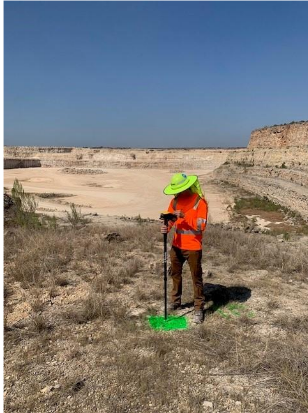
Figure 13: Surveying a ground control point in the Lhoist New Braunfels study area.
