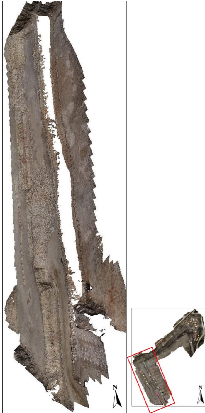
Figure 17: The dense cloud model of the Southwest study area produced in Agisoft Metashape Professional. The second step in the model development process.
