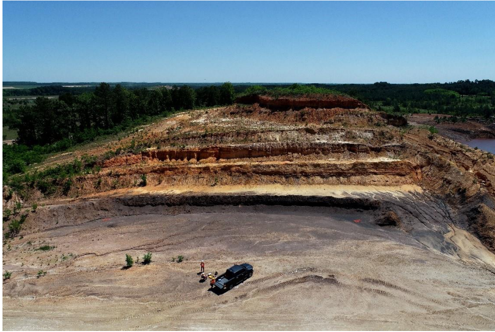
Figure 42: The Alabama Mine study area, Saline County, Arkansas. The 11 bedding units here make up the five mining benches pictured.
