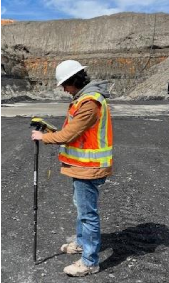
Figure 4: The Trimble™ Geo 7X GPS unit with monopole was used to collect point data along the South Hallsville No.1 Mine highwall in Rusk County, Texas.
