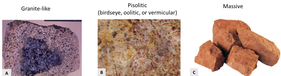
Figure 9: Images displaying different textures of bauxite: (A) granite-like (from Encyclopedia Britannica, 2022, (B) pisolitic (from Van Gosen and Choate, 2021) and (C) massive (from SHE Media collective, 2022).
