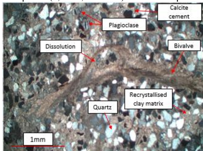
b. Sample 24 (9,885ft, 3012.9m) under plane-polarized light.
