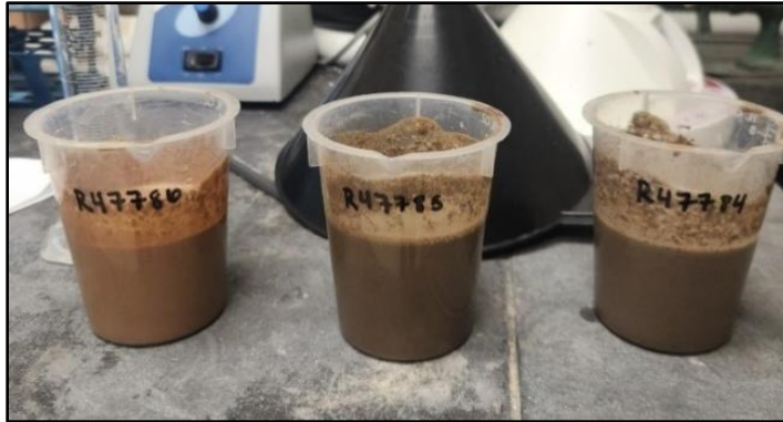
Figure 78. The saturated pastes were created by adding nano pure water to each sample.
