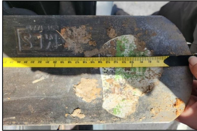
Figure 73. The 15 cm length was measured on the shovel to ensure soil samples were taken at a consistent depth.
