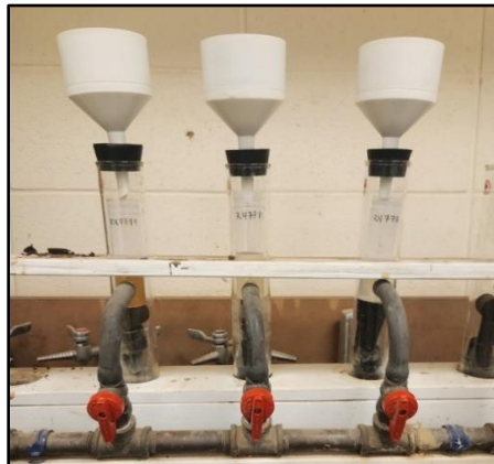
Figure 80. The extraction of the soil samples with a vacuum setup.
