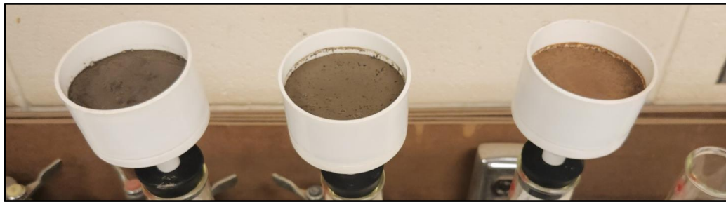
Figure 79. The saturated soils placed in a Buchner funnel lined with filter paper.
