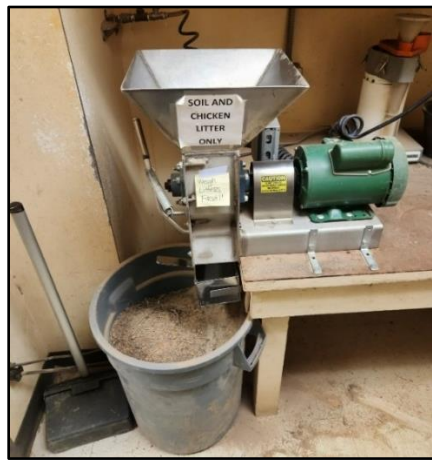
Figure 77. The grinder used to process the soil samples.
