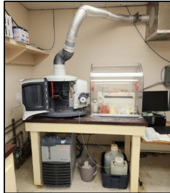
Figure 82. The ICP machine used to identify the concentration of the constituents in the liquid extracts
