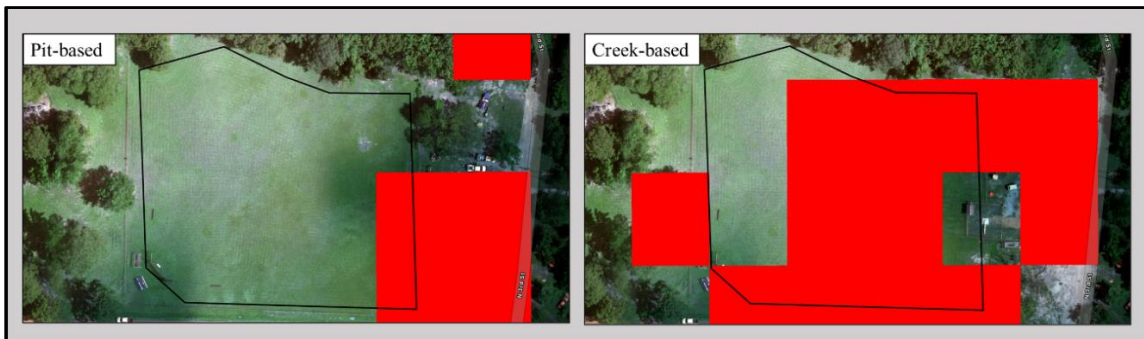
Figure 69. The boundary of the Louann Park site is delineated in black and brine contamination is indicated with red. The pit-based classification is displayed on the left, while the creek-based classification is displayed on the right.
