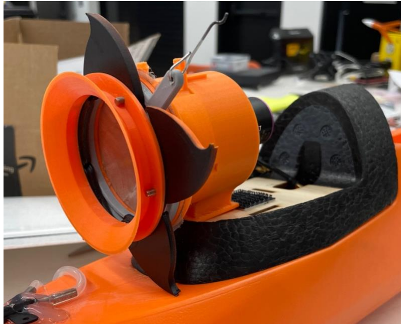
Figure 7. PHASM's syphon. This device is used to syphon cetacean blow mucous onto a collection screen for analysis. The suction maintains the forward directed momentum of the system. The fan and the black colored iris (open) are controlled from the pilot's controller. The iris seals the filter from exposure before and after collection and prevents contamination.
