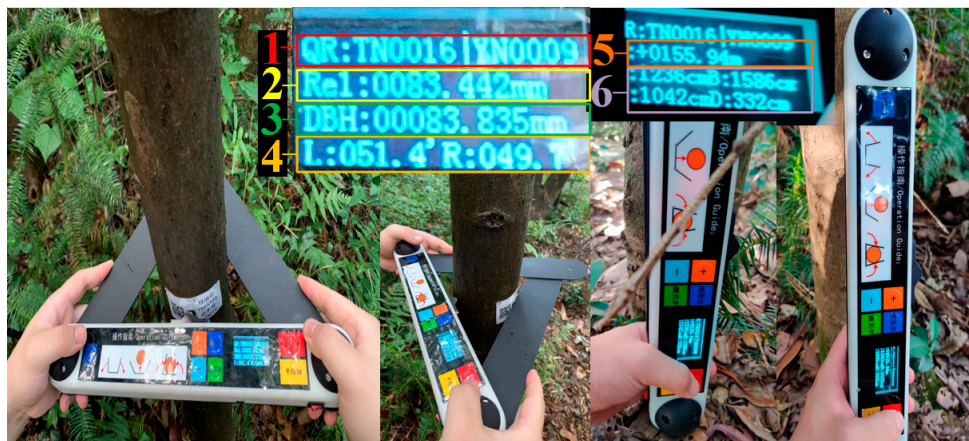
Figure 7. Measurement of a tree. On the display screen, line 1 represents the tree code; line 2, the diameter at breast height (DBH) value of the previously measured tree; line 3, the measured DBH value; line 4, the values of \alpha_1 and \alpha_2 ; line 5, the value of H_n ; and line 6, the values of A_n , B_n , C_n , and D_n .
