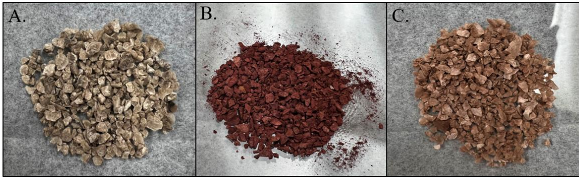
Figure 8.1: Color variations in the salt cuttings from: A. Upper Louann (sample 11,940-11,970 ft (3,639 – 3,643 m)); B. Suture zone (sample 13,530 – 13,560 (4,124 – 4,133 m)); and C. Lower Louann (sample 17,580 – 17,610 (5,358 – 5,367 m)).
