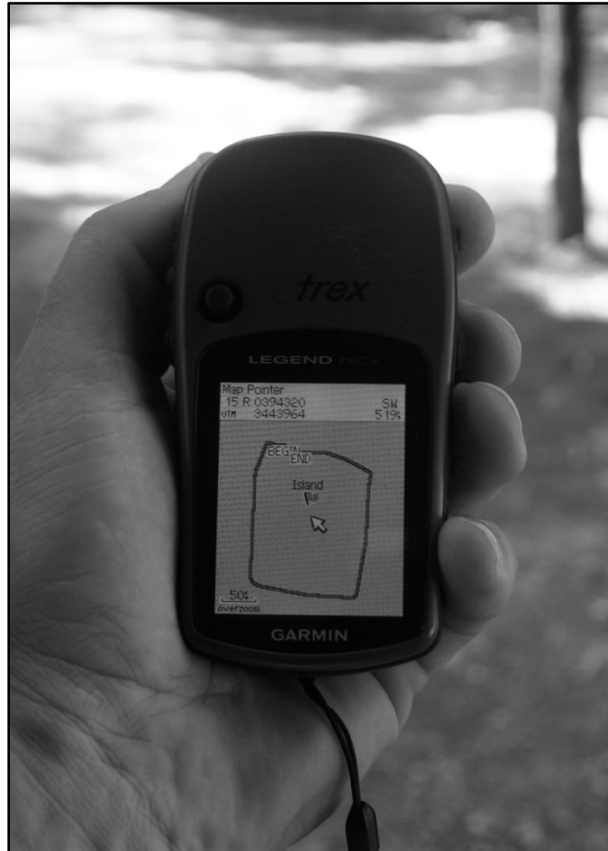
Figure 4. GPS recorded track on Garmin eTrex HCx GPS unit
