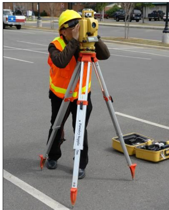
Figure 4. Measuring slope distance with a total station between the top of a light pole and a ground level coordinate identified within a central parking lot on the residential campus of Stephen F. Austin State University, Nacogdoches, Texas.
