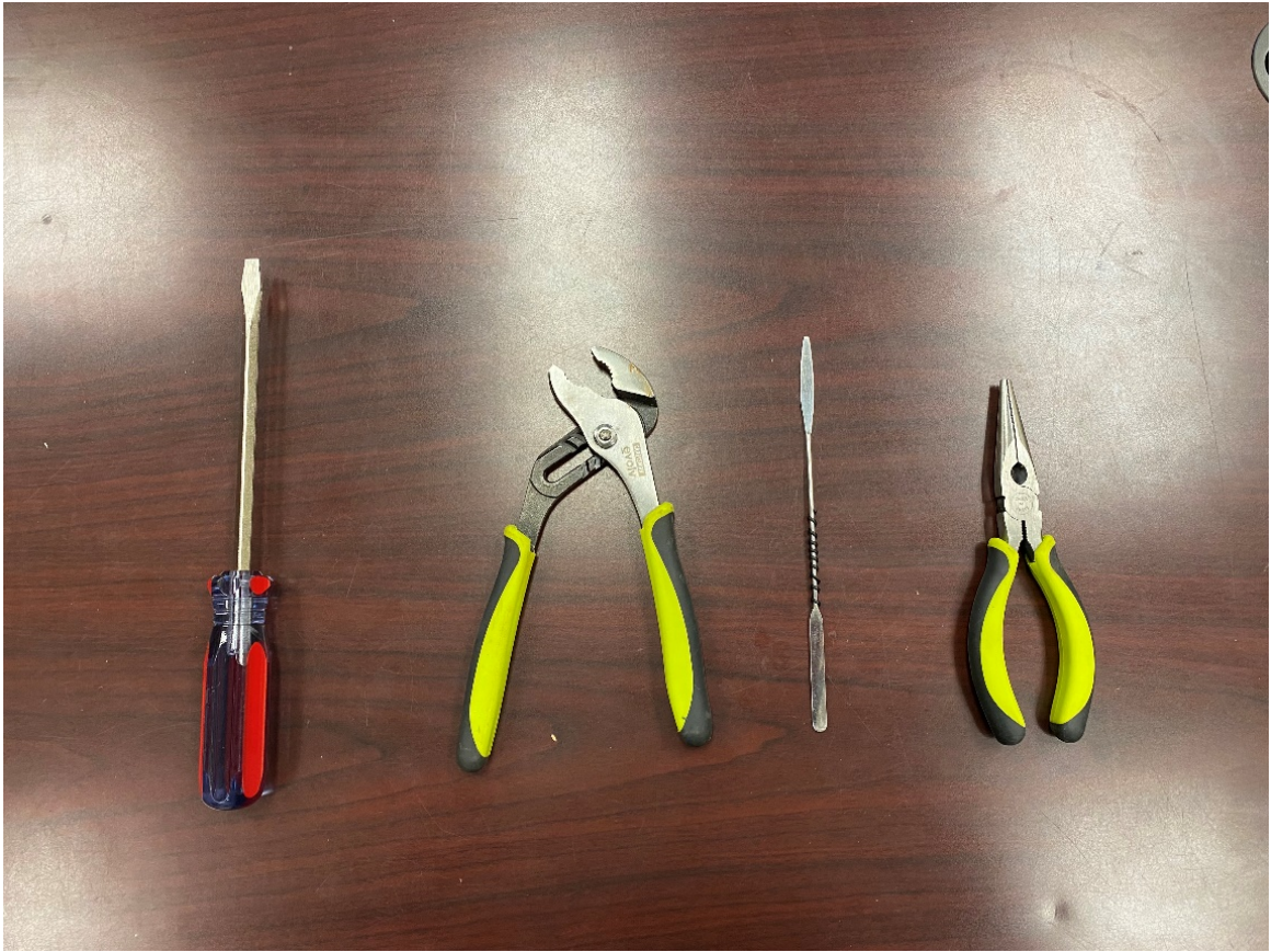
Figure 7. Tools for Removing Posts in Posthole Binders. Primary tools used in the removal of posthole style binders. Photograph taken June 25 th 2021 by Christopher Cotton.
