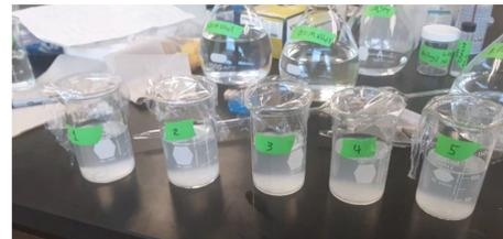
Figure 3. Clay samples ready for ammonia electrode analysis
