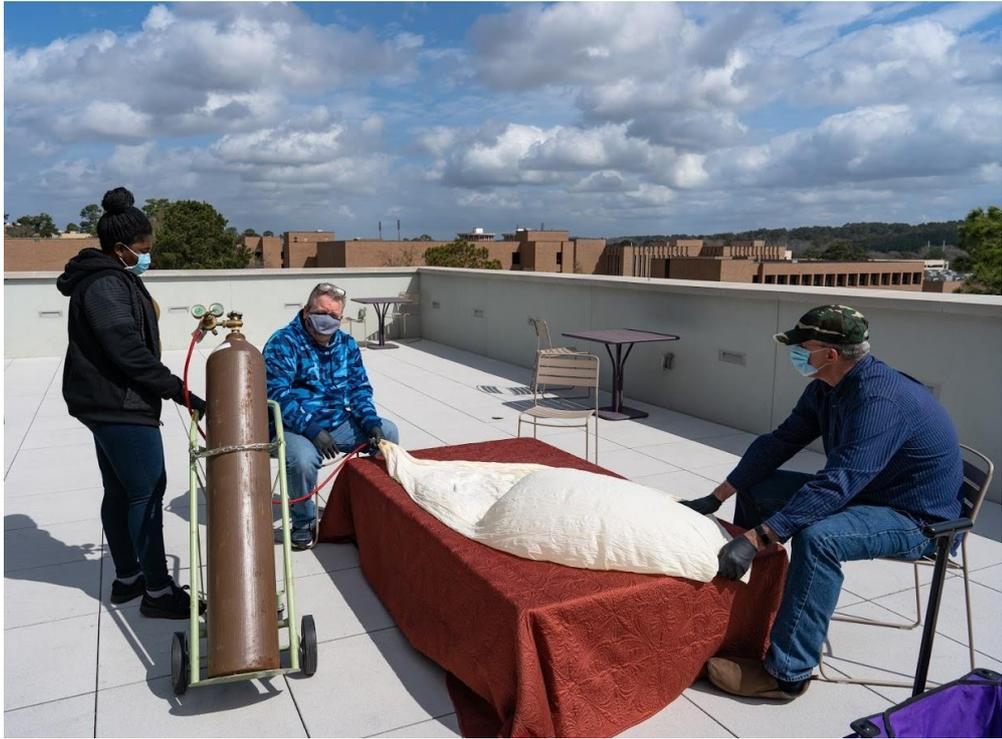
Figure 3.41: The filling of the balloon using Helium.
