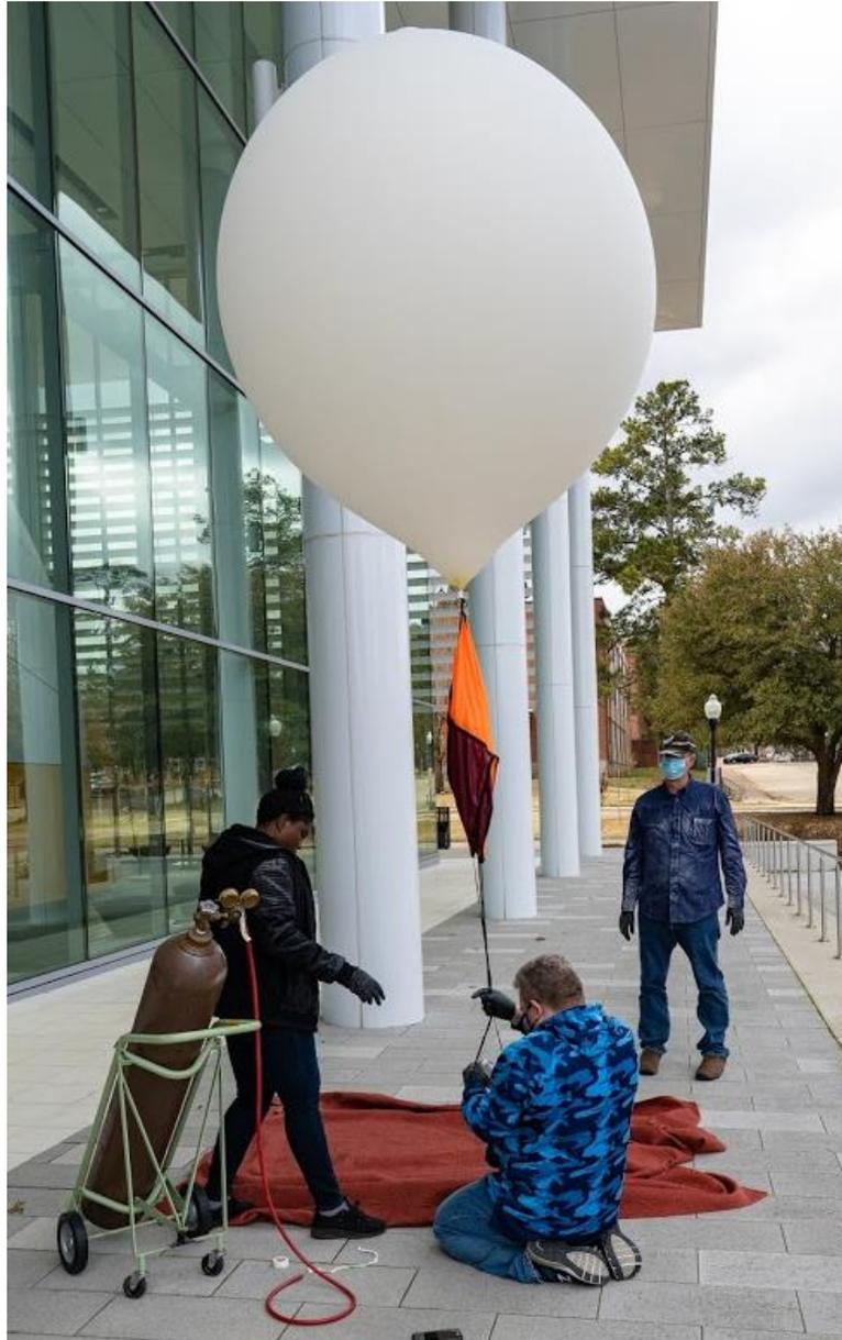
Figure 3.44: Refilling of the balloon after it descended from the observation deck.
