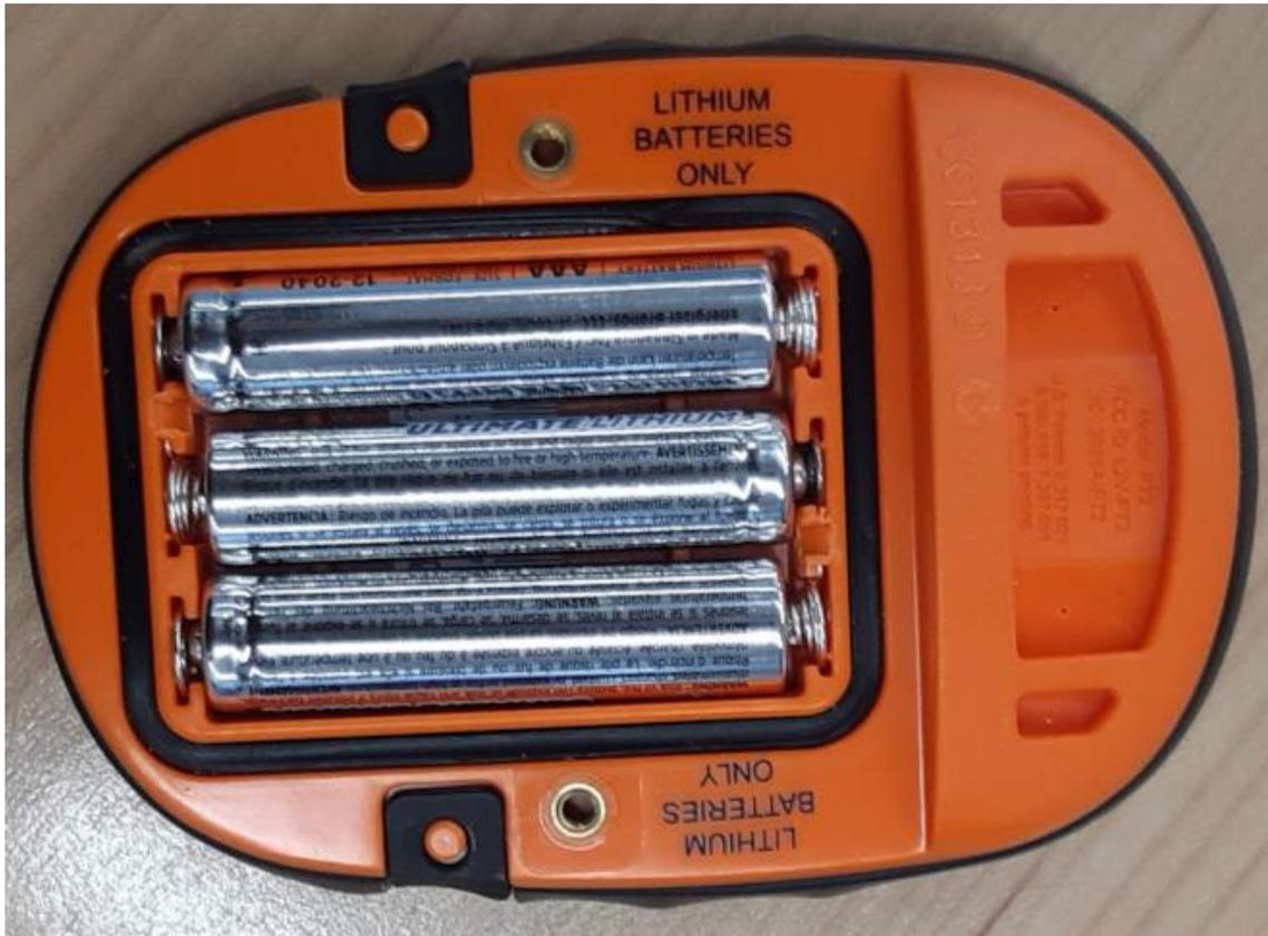
Figure 2.11: SPOT GPS with Lithium batteries.
