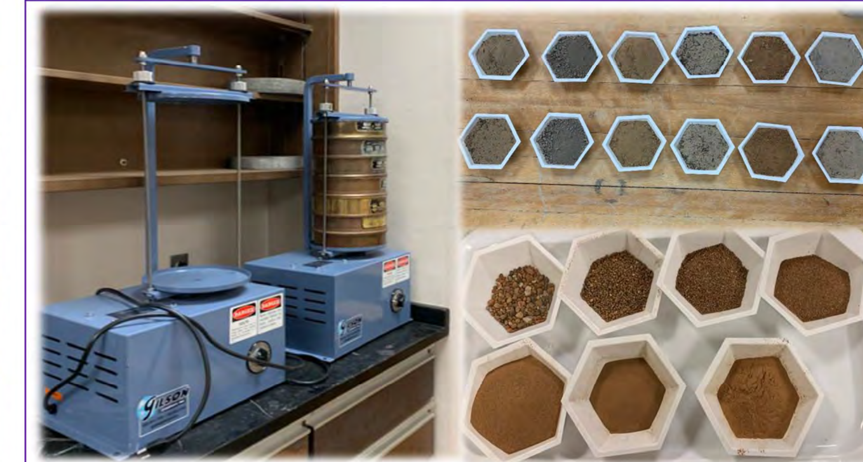
Figure 6: Sieve with sediment before and after. Each sample was put through a Gilson Model SS-15 Sieve Shaker to identify the different grain sizes seen at each location, see Figure 6 .
