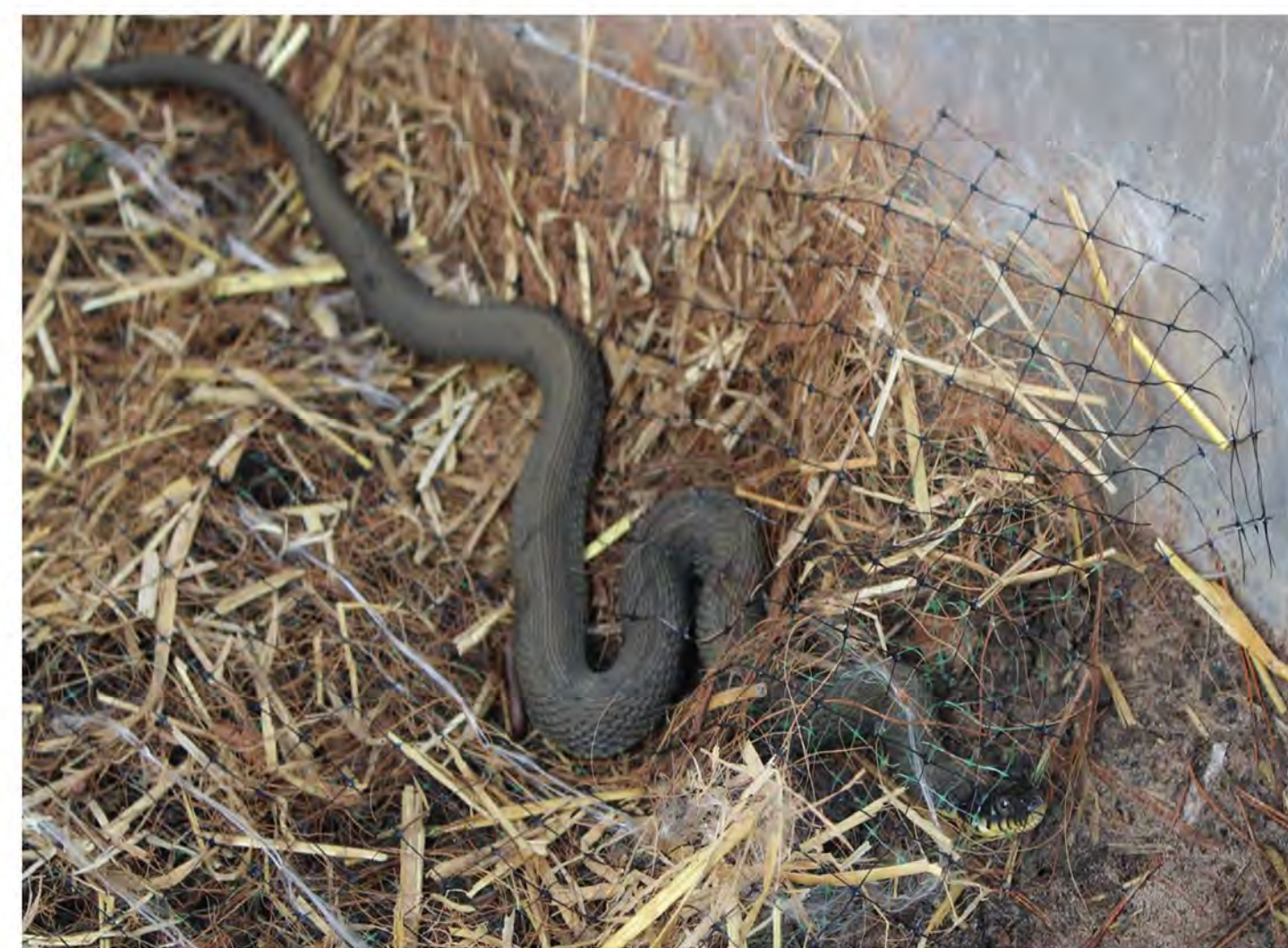
Fig. 1A: Nerodia erythrogaster entangled in Biomac SC (2 layer ECB with fused, polypropylene netting) during snake entanglement trials.
