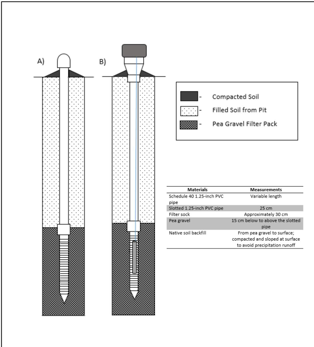
**Figure 5.** Diagram displaying the design of the piezometers used for collection of groundwater data, as well as the design for the piezometer pits. The dimensions of the piezometers and the pits vary based on the location of each point. **Part A** displays the design of a standard piezometer at the site, used for groundwater sampling and measurements. **Part B** displays the design for a piezometer to be used in conjunction with a Solinst Levellogger.
