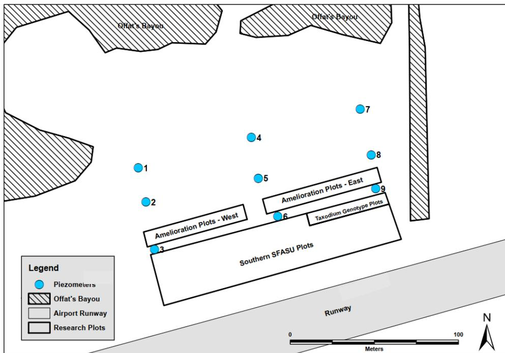
**Figure 1.** Locations of piezometers at the project site. The taxiway of Scholes Field can be seen to the south, while Offat's Bayou can be seen to the north. A channel is visible on the eastern boundary of the site.
