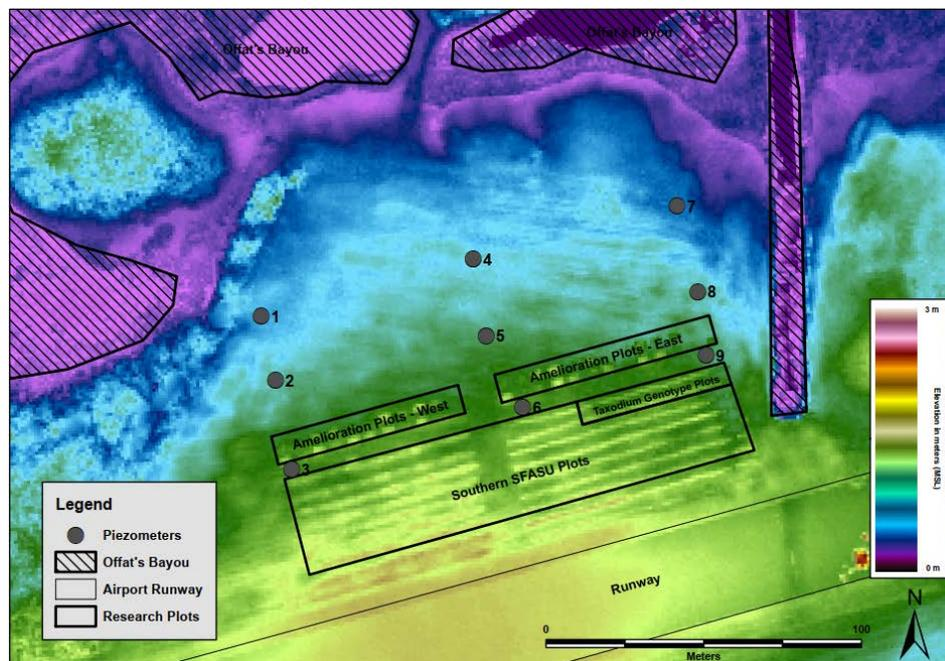
**Figure 3.** Locations of piezometers at the project site. The site map is overlaid on 2017 Houston-Galveston Area Council Light Detection and Ranging (LiDAR) data, accessed through the Texas Natural Resources Information System (TNRIS).
