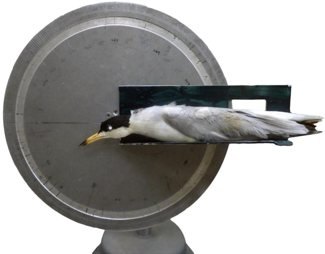
**Figure 4.** The device used for quantifying irradiance. The metal disc can rotate 360°. The spectrometer probe (the white dot centered on the eye of the specimen) runs through the disc, into the side of the specimen's skull, and into the eye socket on the other side.
