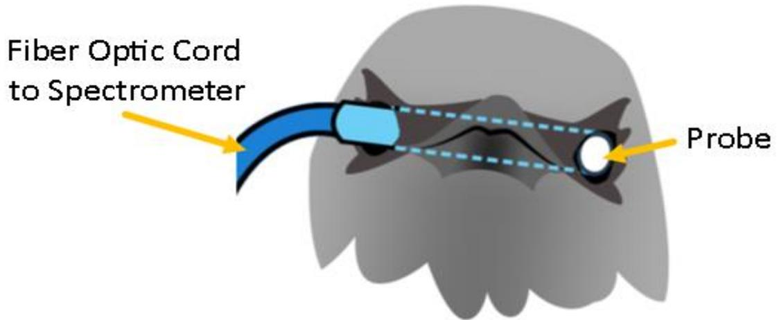
**Figure 3.** The cosine corrector or “probe” inserted through one side of the specimen’s skull so that the probe was placed in the eye position on the other side of the skull.
