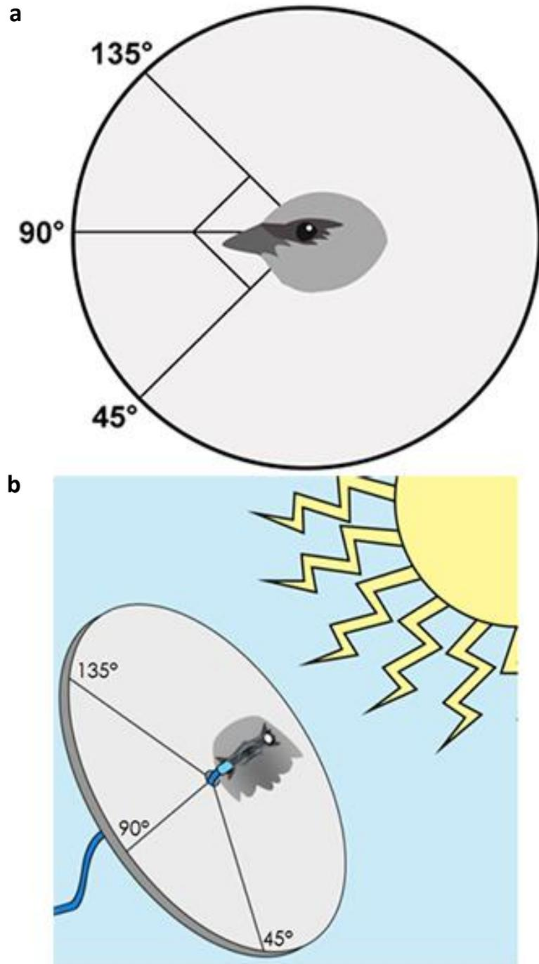
**Figure 5.** Two measurements (with the bird and a baseline reading without the bird) were taken at each tilt ( $135^\circ$ ,  $90^\circ$ , and  $45^\circ$ ) (a) for each bird while maintaining the probe's perpendicular view of the sun (b).
