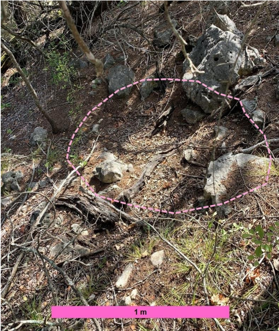
Figure 44: A subsidence feature that was detected by the LiDAR survey and verified during the random point sample survey and agreed with both sets of filters and buffering parameters.
