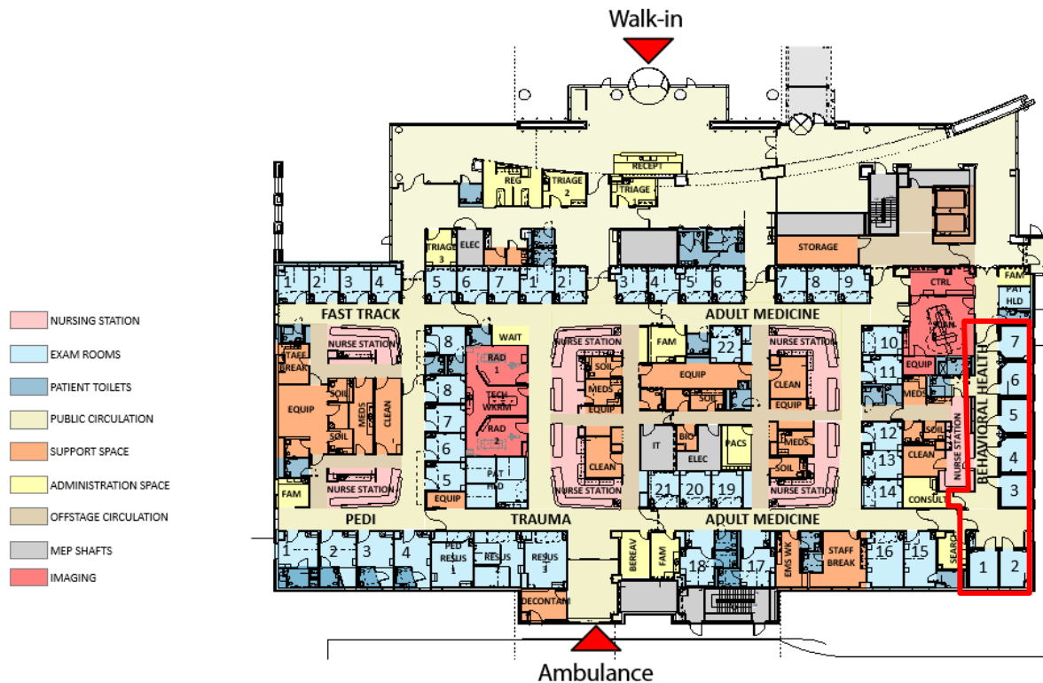
Figure 9. Example of behavioral health treatment unit within the ED (WHR Architects, Inc., 2014).
