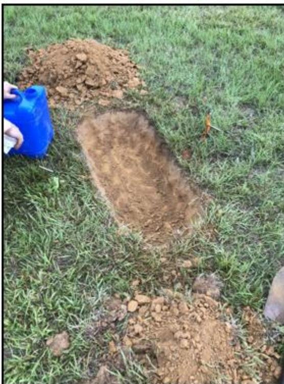
**Figure B 4.** Infiltration pit dug between the 49<sup>th</sup> and 50<sup>th</sup> electrode along survey line one.
