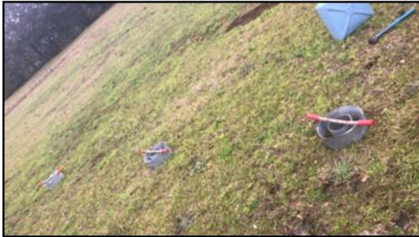
**Figure B 11.** *Three infiltration rings used to conduct the infiltration test at three locations along survey line one. At each of the three locations, three infiltration rings were used and the average rate of infiltration among the three rings was calculated.*
