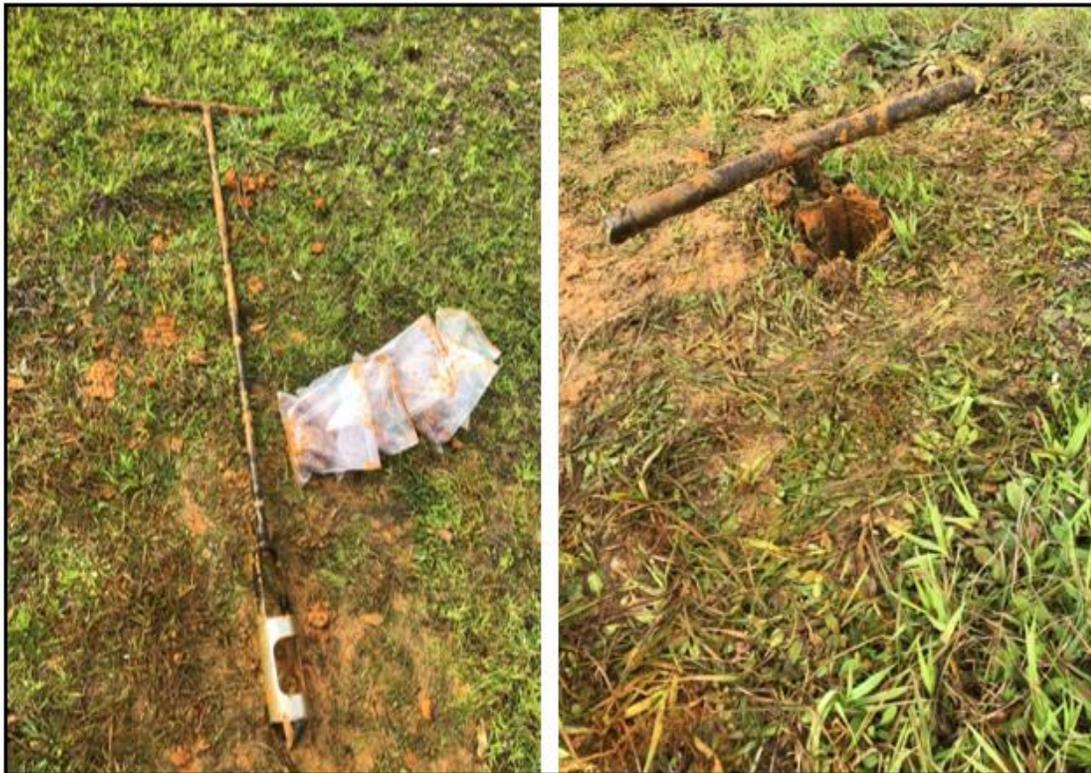
**Figure B 12.** 1.5-meter auger used to collect the three soil cores along survey line one. The samples were collected in ten-centimeter increments and placed in zip lock bags.
