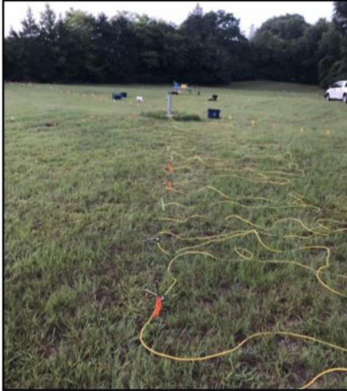
**Figure B 3.** Image of the field setup with electrodes connected to the stakes along survey line one. The flags represent the stake locations for survey line two and survey line three. Seen in the forefront of the image is piezometer one.
