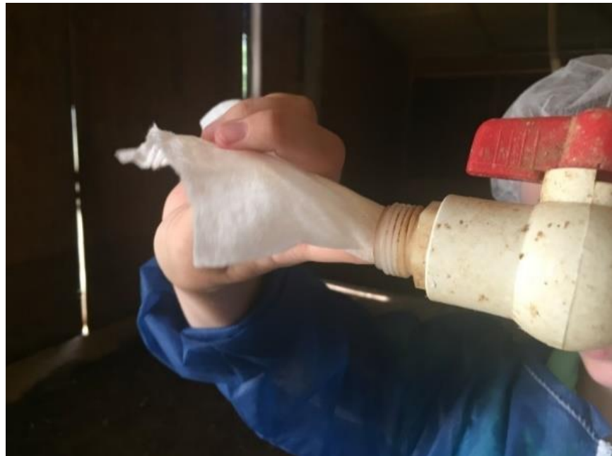
Figure 6. End of Line Sanitization for Swab Sample Collection
