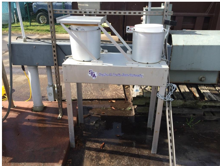
Figure 9. An image of the Precipitation Collector Model 301, in the dry fall sampling position, which was placed at the study site located in the Moody Gardens property in Galveston, Texas.
