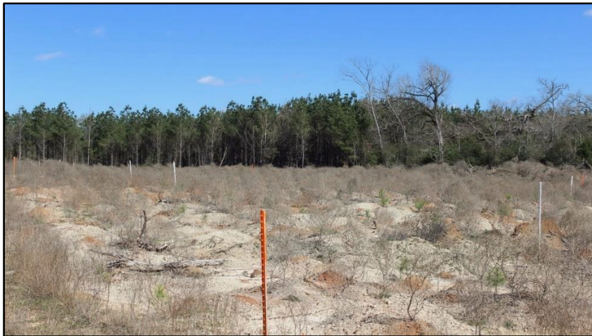
Figure 5. Photo taken in January 2017 of FRA style reclamation plots showing uncompact loose soil piles.
