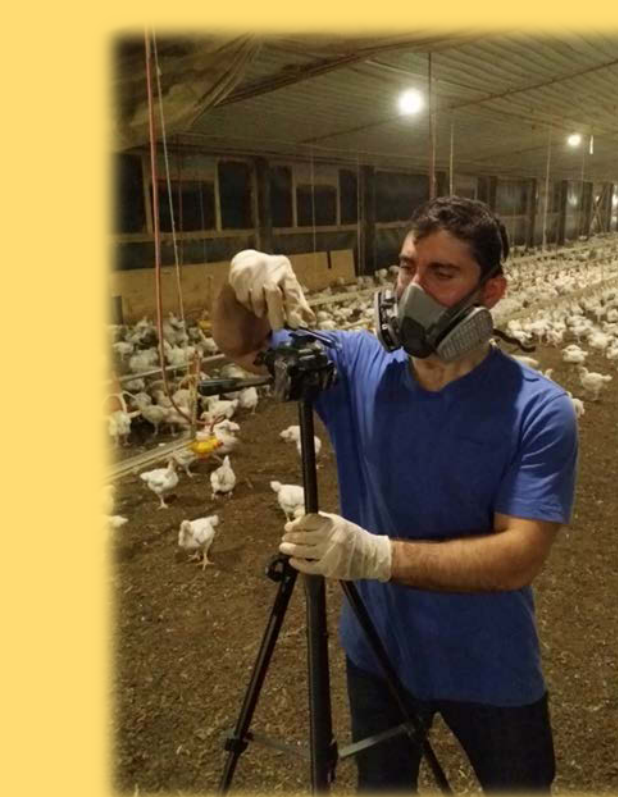
Setting up a Colorimetric NH 3 Sampler Tube Inside One of the Chicken Houses for Aerial Exposure Sampling.
