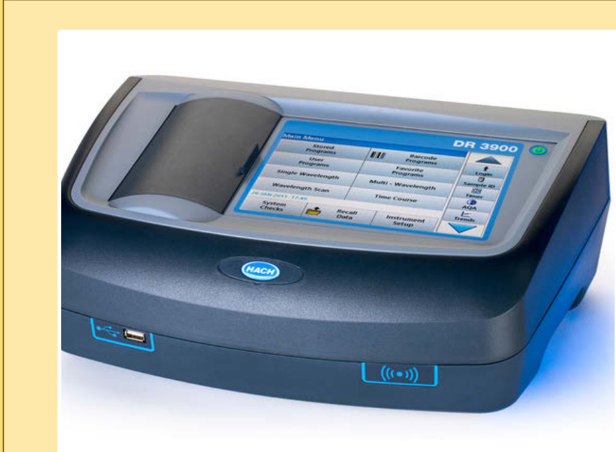
DR 3900 Benchtop Spectrophotometer with RFID® Technology that was used in the study to measure NH 3 concentrations. The spectrophotometer measures the amount of light of a specified wavelength which passes through a medium. According to Beer's law, the amount of light absorbed by a medium is proportional to the concentration of the absorbing material or solute present.
