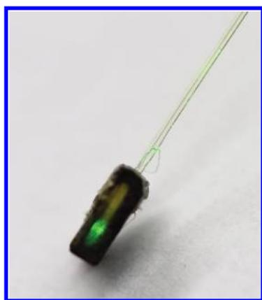
**Figure 2.** Image of the HC-580 fiber inserted into the silica cap (length = 2.38 mm, bore diameter = 0.38 mm). Green light exited the distal end of the fiber. The absorption of light by the sensitizer occurs in the PVG cap.
