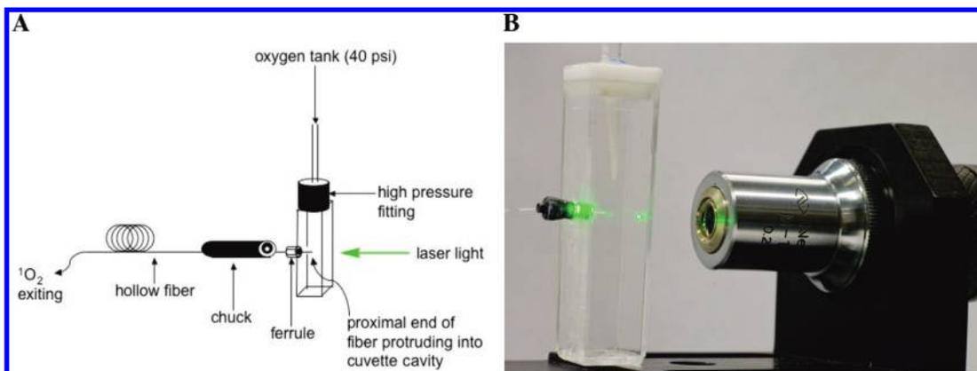
**Figure 1.** (A) A schematic drawing showing the compressed oxygen-to-fiber coupling and the use of a modified cuvette. Oxygen gas is delivered through a pipet at the top of the cuvette and enters the proximal end of the fiber to the left, which is protruding into the cuvette cavity. (B) A portion of the experimental setup showing the LED, the 10× objective, and modified cuvette in which green light is focused into the fiber.
