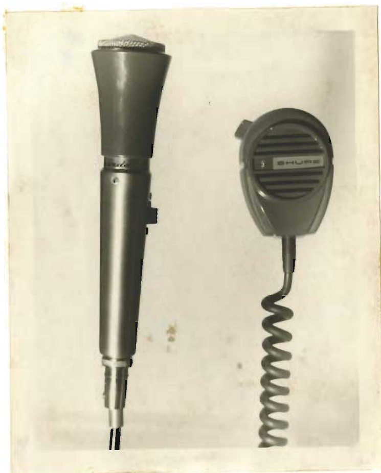
Figure 4. Omnidirectional studio stalk type microphone (left), and palm type field microphone (right).
