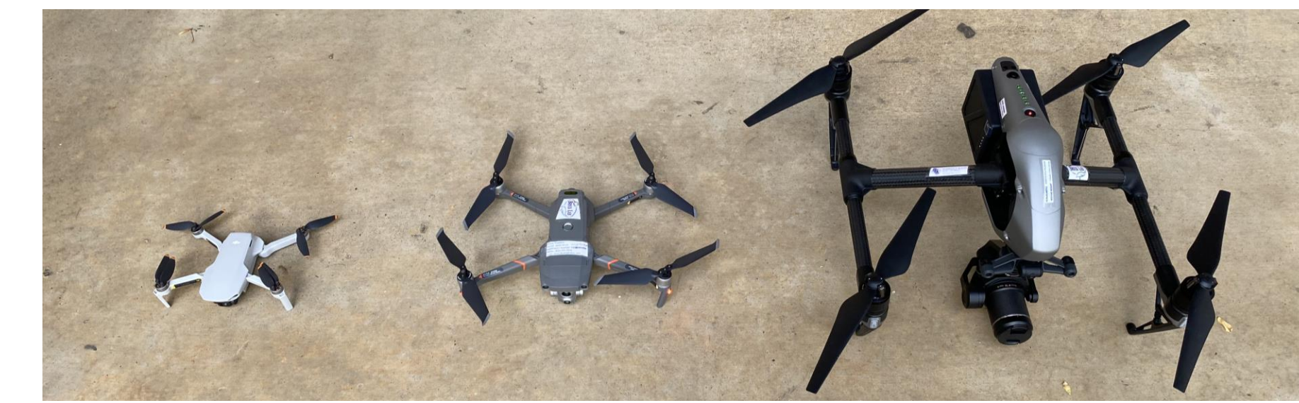
Figure 9. (Left to right) DJI Mini 2, (quiet, but more readily subject to 'blow away'), DJI Mavic 2 Enterprise Advanced (thermal camera \pm 2^\circ\text{C} temperature measurement accuracy), DJI Inspire 2 (wind resistance, can handle ocean air currents, high resolution camera, dual pilot controls, standard on marine mammal research).
